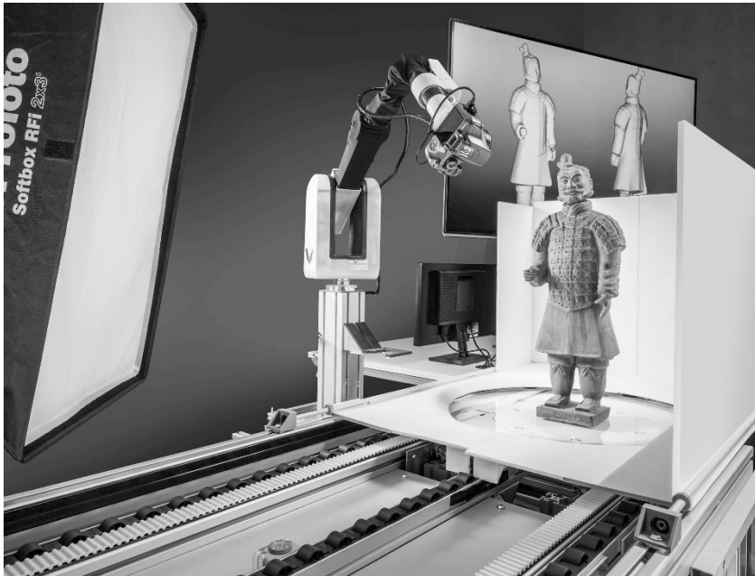
Fig. 3.3 CultArm3D: lightweight robotic arm with a 24-megapixel camera mounted to the end effector next to a turntable with a white two-part folding studio box (Fraunhofer IGD)
