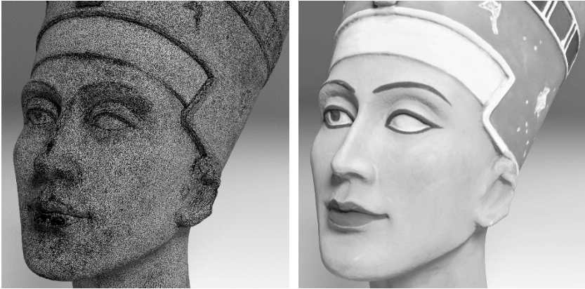
Fig. 3.4 Left: 3D reconstruction of a replica of Nefertiti – mesh; right: 3D reconstruction of a replica of Nefertiti – final color-calibrated 3D model (Fraunhofer IGD)
