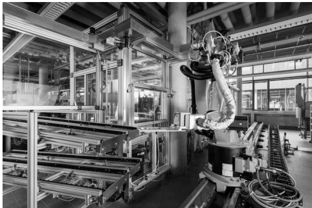
Fig. 13.4 View of Fraunhofer IFAM’s assembly line for the digital functionalization of FRP components (Fraunhofer IFAM)
