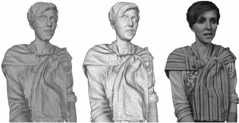
Fig 4.3 3D person reconstruction; left : 3D geometry as originally reconstructed point cloud; center : 3D geometry as reduced wireframe; right : textured model with projected videos from the multi-camera system, source [7] (Fraunhofer HHI)
