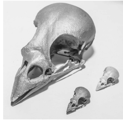
Fig. 10.4 Reproduction following scanning of a bird skull in original size and at ten times actual size (Fraunhofer IWS)
