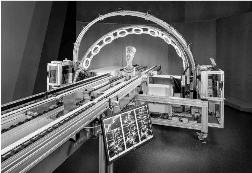
Fig. 3.2 CultArc3D: two hemispherical rotating arches, one with cameras, the other with ring light sources (Fraunhofer IGD)
