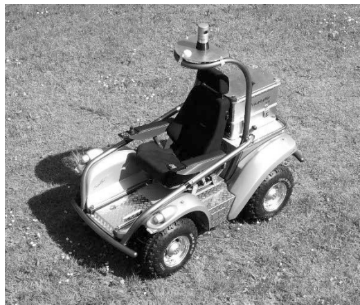
Fig. 14.6 The IOSB.amp Q2 autonomous mobile robot is able to support rescue workers in quickly gaining an overview of the situation. (Fraunhofer IOSB)
