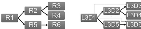
Fig. 3.11 Left: 3D data from CAD systems is usually depicted as a linked hierarchy of resources; right: from the point of view of the application, the 3D data is made up of a linked network of 3D data. (Fraunhofer IGD)
