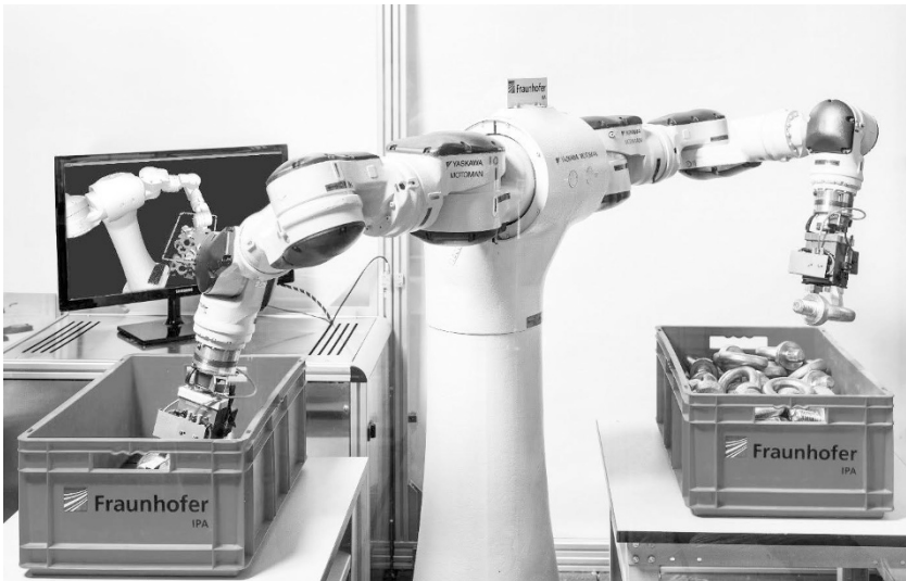
Fig. 14.3 Machine learning processes optimize robot-based systems for bin picking. (Fraunhofer IPA/photo: Rainer Bez)
