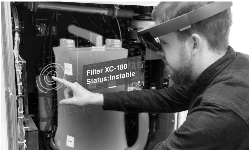
Fig. 3.10 Demonstrator of Augmented Reality-assisted maintenance with HoloLens (Fraunhofer IGD)
