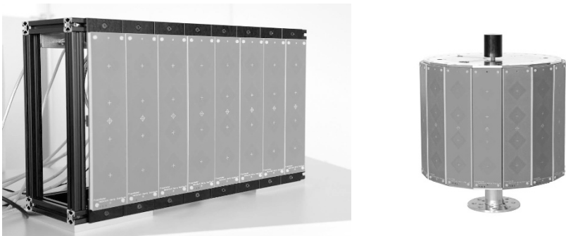
Fig. 7.4 Examples of a 64-element planar (left) and 128-element circular antenna array (right) for massive MIMO antennas for new radio bands at 3.5 GHz (Fraunhofer HHI)
