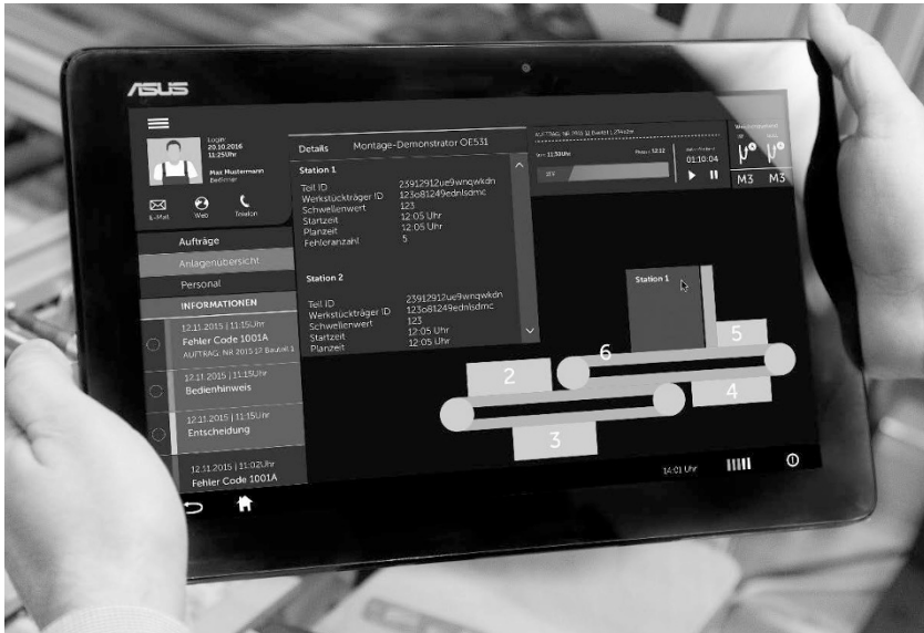
Fig. 12.10 Role-specific and person-specific visualizations (plant overview, job details, notifications, directions) [20] (TYP4 Photography + Design, Phillip Hiersemann, www.typ4.net )
